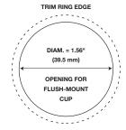
Figure 2. Use this template to flush-mount a Kappa10.1t tweeter.
